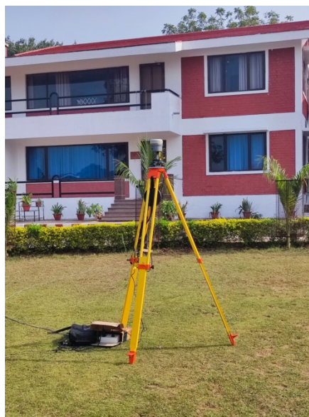
Figure 14: Base Station Setup
