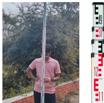
Figure 11: A man holding Levelling Staff
