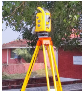
Figure 8: A Tripod (with Total Station)
