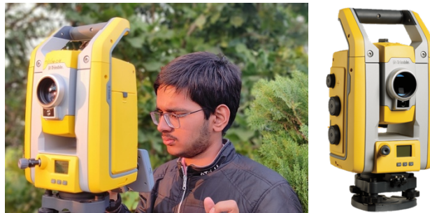
Figure 5: A man using Trimble S5 Total Station
