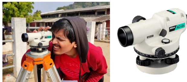
Figure 10: A man using Auto Level
